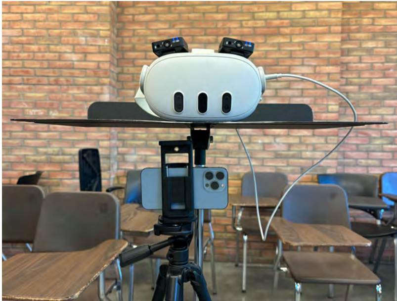
Figure 10: Data collection setup: A Meta Quest 3 with 2 attached Rode Wireless GO II microphones captures the mono audio, while a stationary iPhone records a third-person view of the scene.
